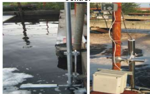
Control of the dissolved oxygen concentration in a wastewater treatment plant
