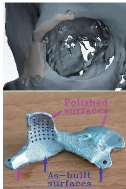
Fig. 4. Facial customized implant designed and fabricated made of Ti-Gr.
