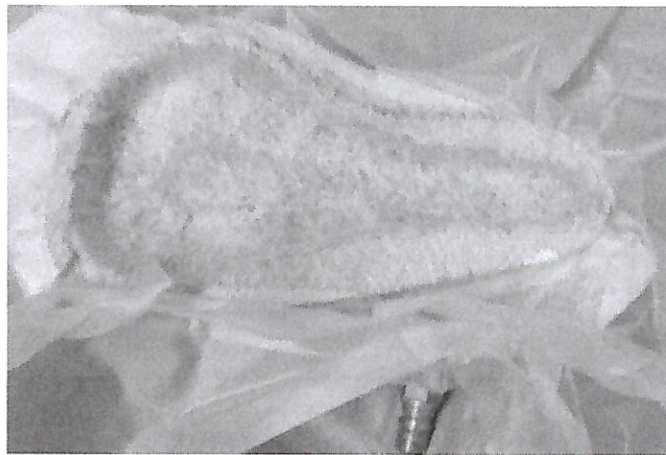
Fig. 10 – Applying vacuum pressure through mold and composite material.
