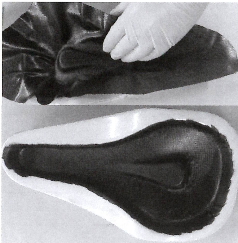
Fig. 9 – Application of CFRP layers on the mold.
