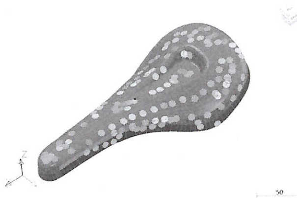
Fig. 14 – Points acquired on CFRP seat post.
