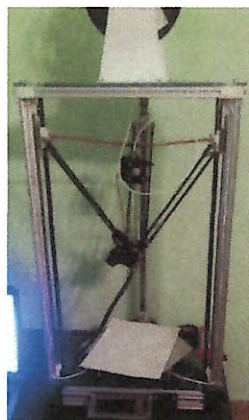
Fig. 10. The prototype of the Delta printer
