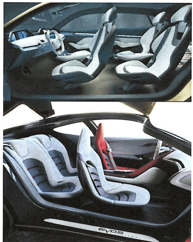
Fig. 2 Monocoque car seats [2, 3]
