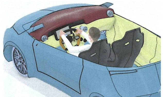
Fig. 8 Asymmetrical seats in the body of the prototype
